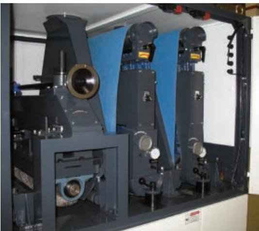
**Figure 3** With its new slag grinder, Vac-Con no longer has to worry about manual grinding to remove slag, only manually feeding parts into the new equipment. Moving from right to left, plasma-cut parts progress underneath two abrasive rollers and then to a wire brush that rotates in the direction opposite of the material flow.
