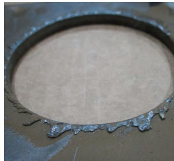
**Figure 2** Any fabricating shop that works with older plasma cutting equipment is familiar with the slag left over from a cut.
