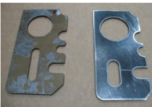
**Figure 4** Vac-Con's slag grinder proved effective in removing slag from plasma-cut parts.
