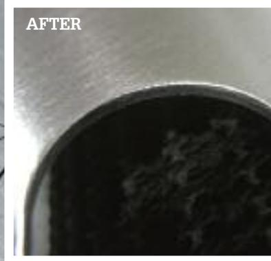
This laser-cut mild steel was processed with a Puma series deburring and finishing machine.
